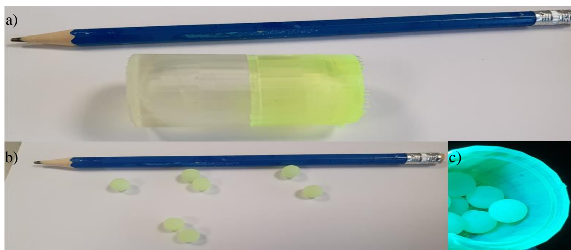
Figure 4. a) Example of photoactive 3D printed milling jar (right half), b) balls, and c) their fluorescence under long UV irradiation.
