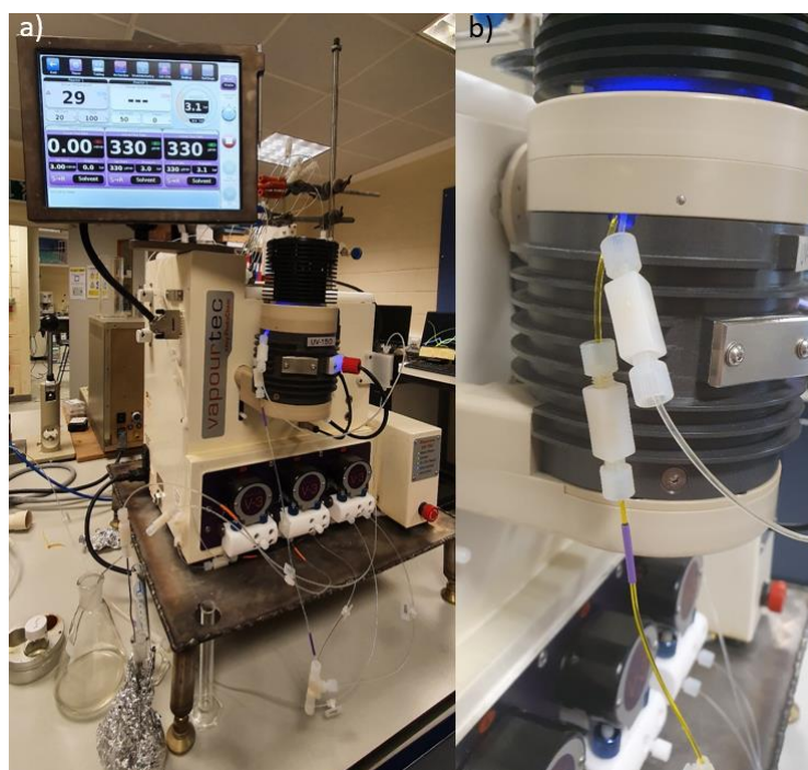
Figure S5. Photographs of the flow reaction setup (Method B). a) Vapourtec E-series equipped with the Photochem UV-150 module. b) Close-up photograph of the UV-150 reactor during operation. The tube on the left containing the yellow-coloured solution is flowing towards the reactor. The tube of the right is the outlet of the reactor, and as it can be seen, the fluid is colourless, indicating that the reaction is complete.
