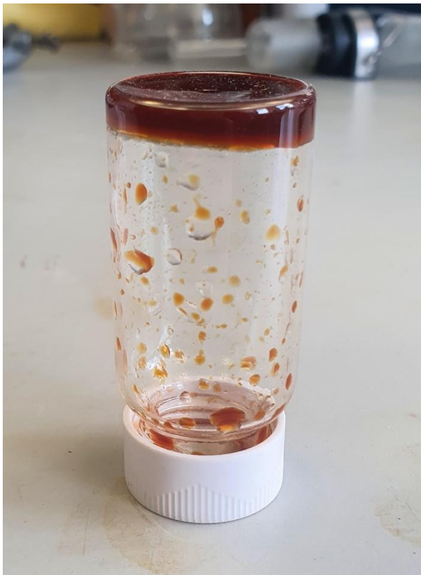
Figure S4. A gel was formed after 2eq. of TEA were added in a solution containing AlaHA and 3eq. of \text{Fe}^{3+} dissolved in \sim 1\text{mL} of DMSO. Similar behaviour was observed in \text{Ga}^{3+} complexes after TEA addition, forming clear gels. In general, it was observed that gelation was generally more pronounced the more TEA was added.
