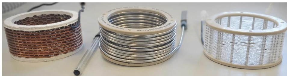
Figure 5. Photographs of copper, stainless steel, and PTFE coil reactors (from left to right).
