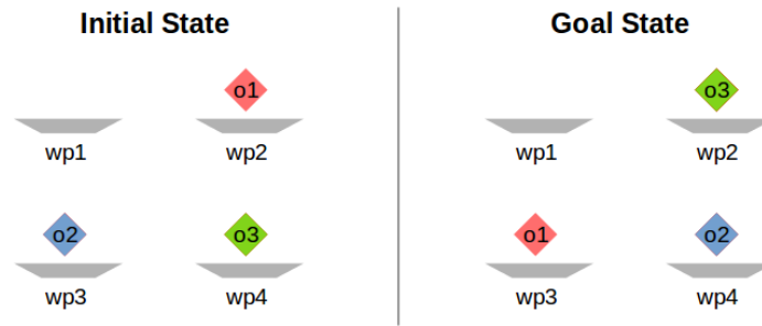
Figure 3.3: A problem of Robot Fetch which requires the robot to start by placing any of the objects, o1 , o2 , or o3 , at the location wp1 instead of their respective goal locations as none of their goal locations are empty.
