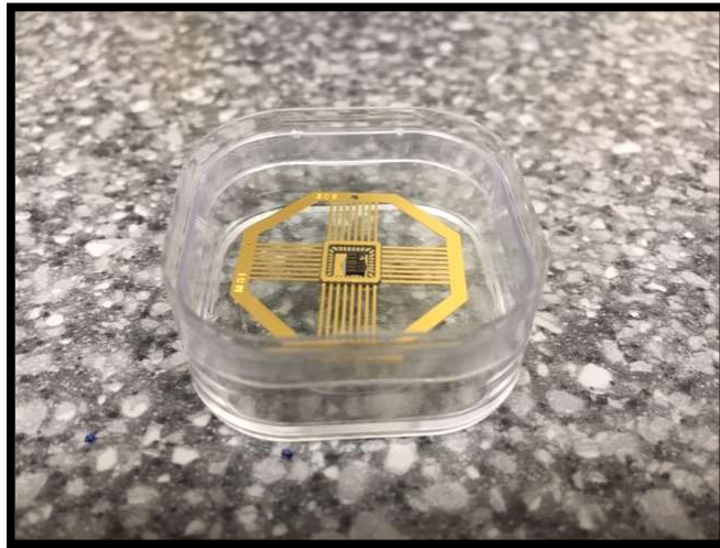
Figure 5.6. Ge-on-Si SPAD chip mounted onto a gold electrical package using silver conductive paint, ready to be wire bonded for further characterisation.
