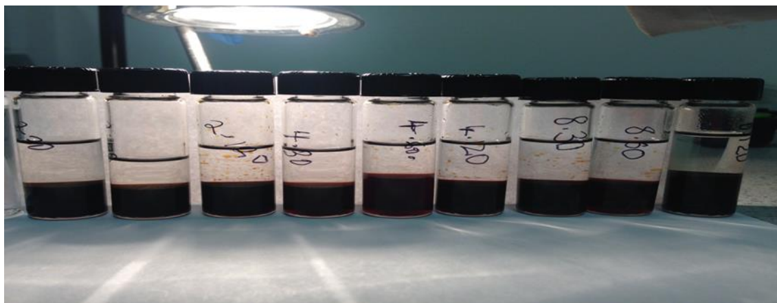
Figure 6-3: Liquid to liquid extraction of the black liquor from the birch wood sample.
