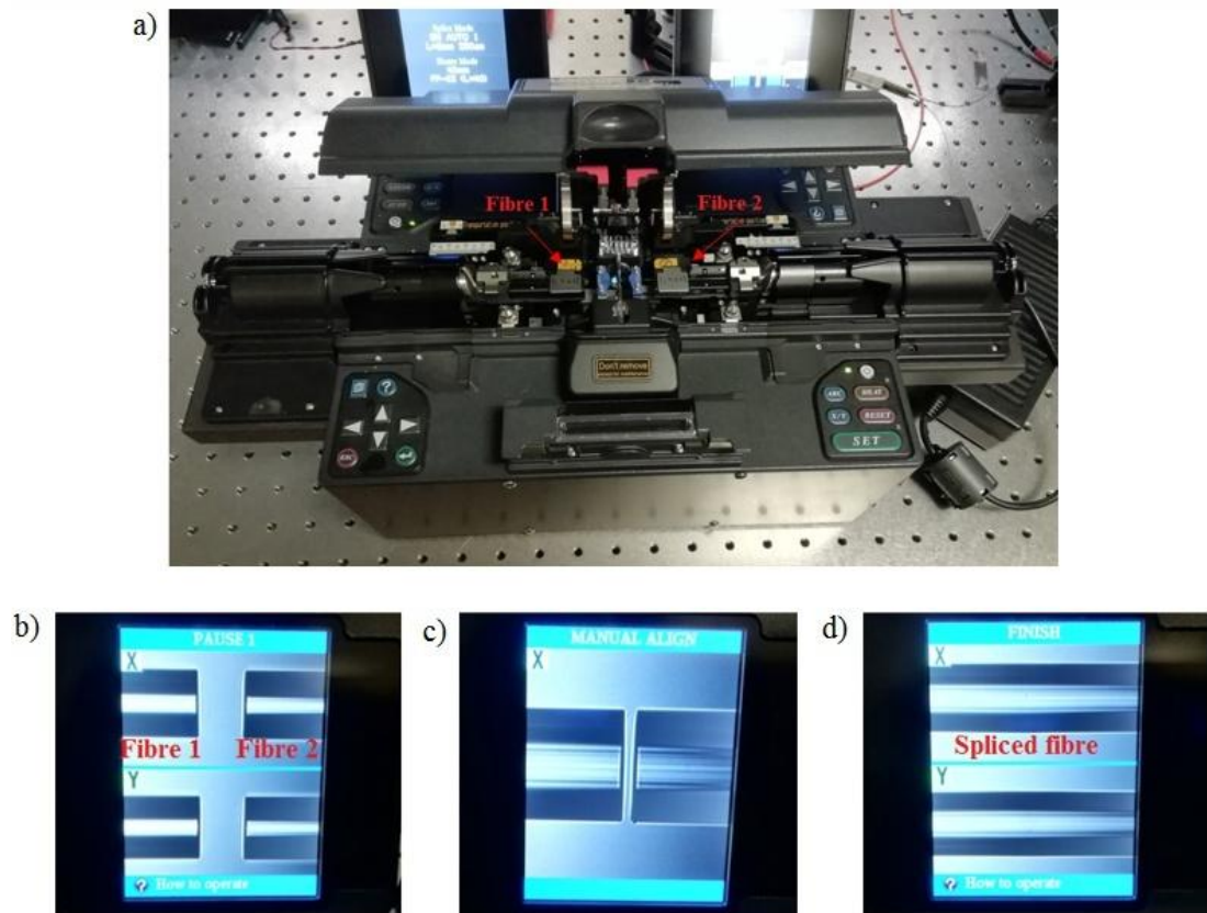
Figure 4. 24: a) Photograph of the fusion splicer used in this thesis. b) Screen showing the cross-section of two single-core fibres of 125µm cladding diameter, placed inside the splicer, before the splice. The X and Y indicate the respective cross sections of the fibres. c) The two fibres are manually aligned along their core axis. d) Image of the new fibre after the splice of the two single fibres.
