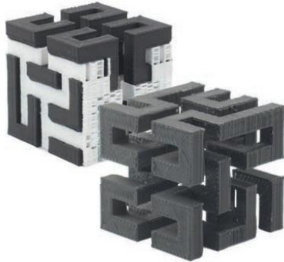
Figure 2.6: FDM printing with white support material (back) and then removed (front) revealing a Hilbert cube. [27]
