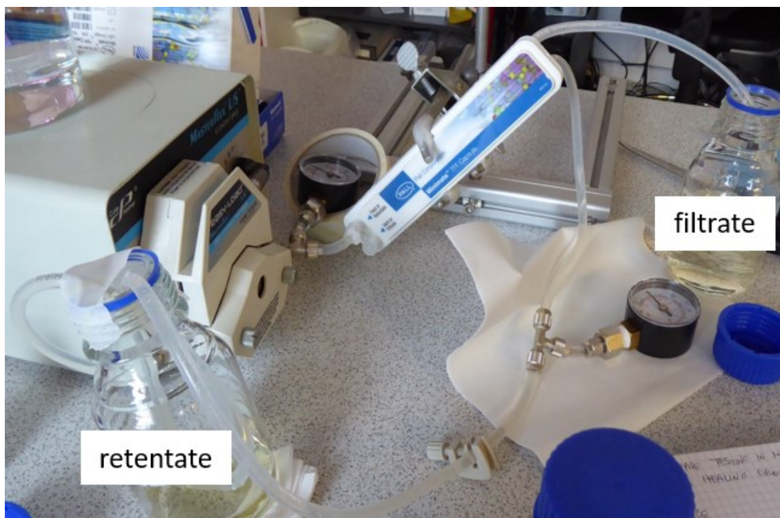
Figure 2.5. Tangential flow filtration setup. The sample starts its journey from the “retentate” bottle, the liquid was pumped in the 500 kDa or 30 kDa cartridge measuring the pressure in order not to damage the filter. The filtrate was collected in a separate bottle and the retentate pressure was controlled with a clip in order to increase the flow to the filtrate bottle. The process was run for several min, until the retentate volume was too low for the system.
