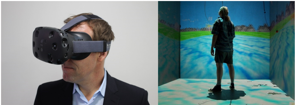
Figure 2.1: Virtual Reality Examples: (Left) HTC Vive headset that is tracked in 3D space. (Right) A CAVE where the displayed image is projected onto a surrounding surface from the user's perspective.
