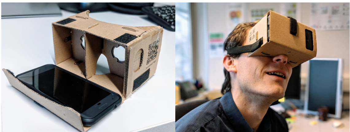
Figure 2.3: (Left) Shows how a mobile phone is placed as the display for Google Cardboard head-mounted display. (Right) Shows the placement of the Google Cardboard display in use.
