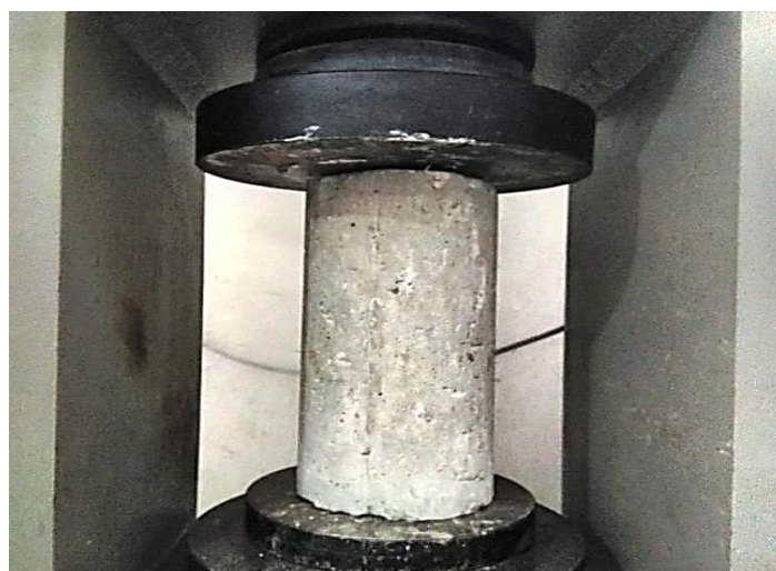
Figure 8. Placement of concrete cylinder in compression testing machine.
