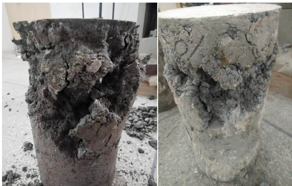
Figure 9. Failure mode of concrete cylinders with recycled plastics after compression test.
