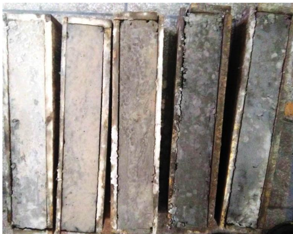
Figure 16. Simple concrete beams for flexural strength test.
