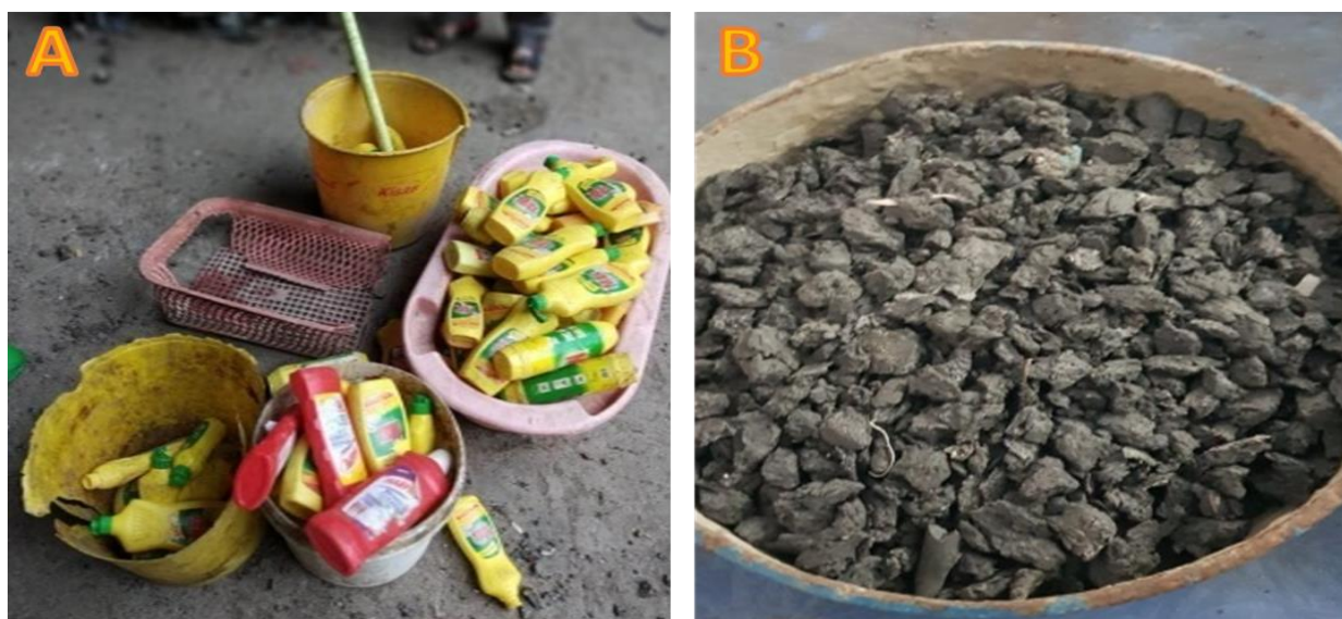
Figure 1. Discarded plastic scrap on left (A) and its conversion into HDPE shown on right (B).
