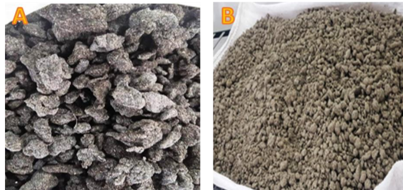
Figure 4. (A) E-waste and (B) HDPE aggregates after sand coating.
