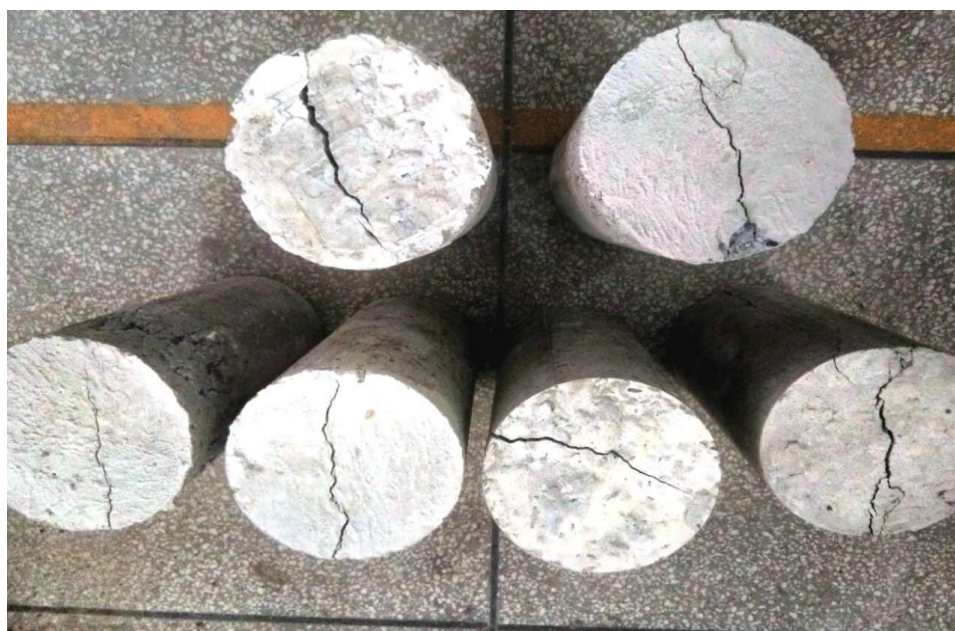
Figure 13. Failure mode of concrete cylinders with recycled plastics after split tensile strength test.
