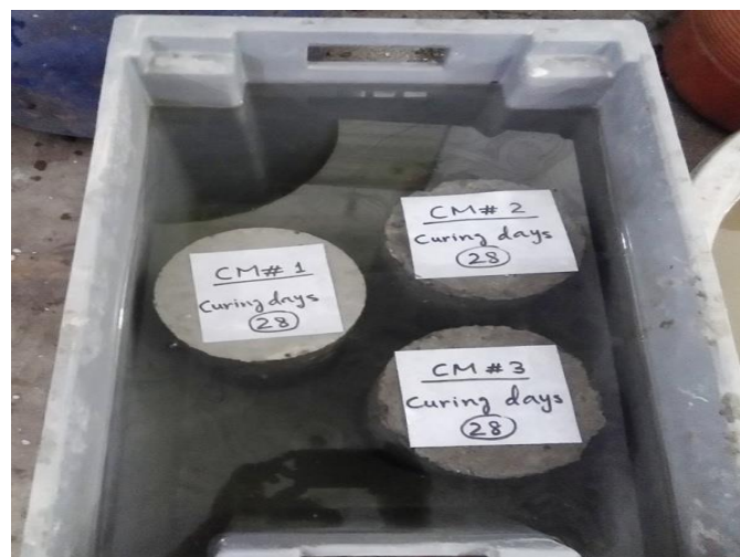
Figure 7. Placement of concrete cylinder in water tab for 28 days curing.
