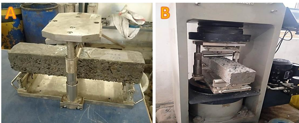
Figure 17. Central point loading assembly for flexural strength test on left (A), and beam with central point loading assembly placed in the flexural testing machine on right (B).
