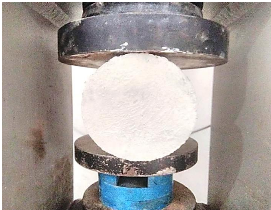
Figure 12. Placement of concrete cylinder in compression testing machine for split tensile strength test.
