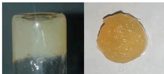
Figure 2. Physically crosslinked hydrogels formed in the equimolar mixtures (1:1) of chitosan hydrochloride and pectin.
