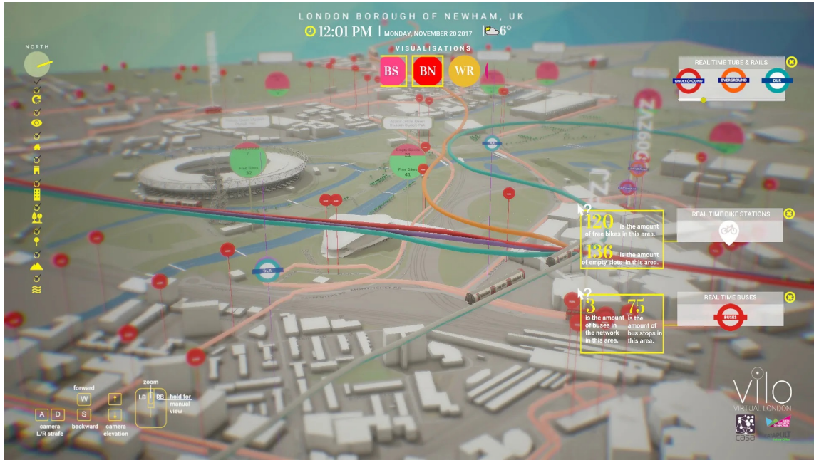
FIGURE 4: Simulation of reality through DTs: ViLO model showing live sensor data on infrastructure equipped with VR and AR [28]. 3D urban modelling and virtual urban static and mobile objects reflecting the streamlining of the real data of CPSs are blended and this scene is augmented with information/knowledge/wisdom from real world activities for effective decision-making.
