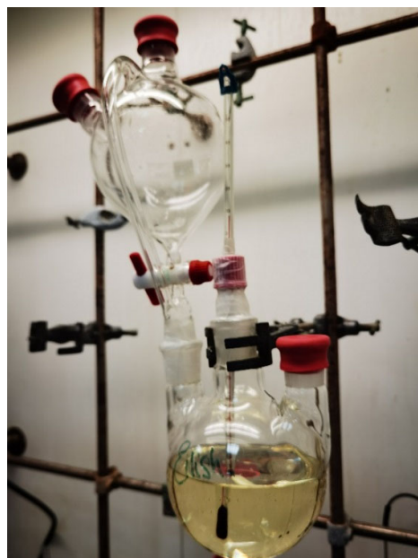
Figure 21. The set up for ethyl 4-methyl-2-oxopentanoate ( 58 ) preparation under dry condition ( N_2 balloons not shown).
