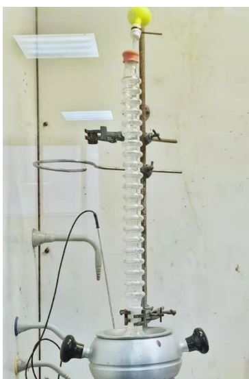
Figure 17. The set-up of the procedure to synthesis L -leucinamide hydrochloride. The condenser is stoppered with a septum and a nitrogen balloon on the top to form a closed system with controlled building pressure.
