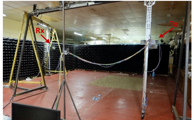
Fig. 1. The GBSAR laboratory in a bistatic configuration.
