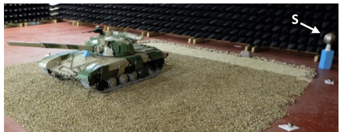
Fig. 3 Target scene, consisting of a Quarter scale T72 tank model on gravel, and reference sphere “S”.
