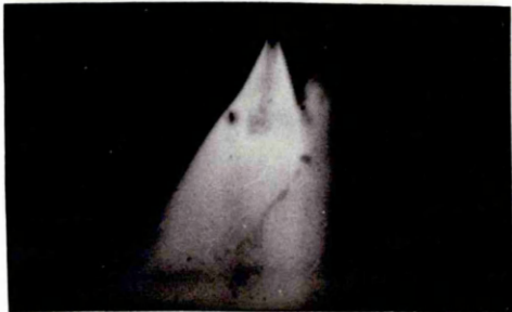
Figure 89. Spatter mechanism of stream spray transfer. Time lapse between frames is 0.43ms, 290A, 1.2mm dia. wire.
