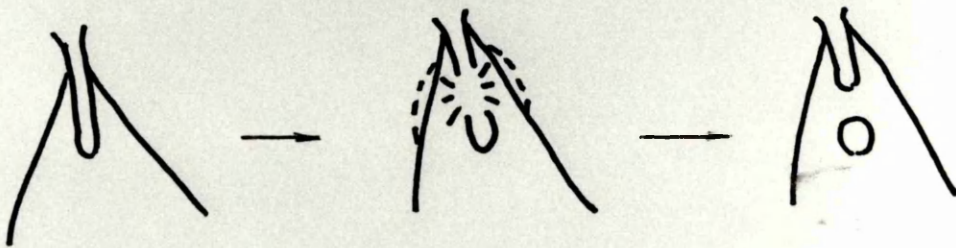
Figure 55. Schematic diagram of drop detachment mechanisms.
