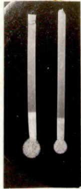
Figure 91. Globular transfer, 1.2mm dia. wire, 91A and 147A.
