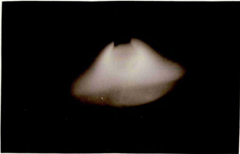
Figure 31. Globular transfer in MIG welding. 1.2mm dia. mild steel wire, Ar + 5% CO 2 , 200A.
