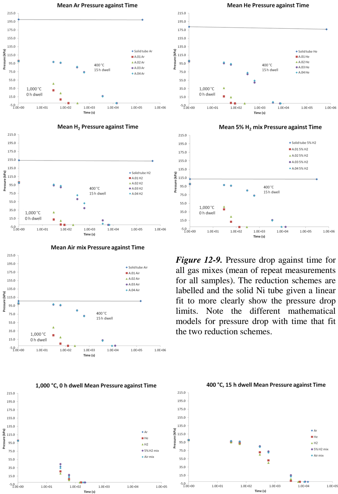
Figure 12-10. Pressure drop against time for all gas mixes (mean of all four measurements pre anode type) divided by reduction scheme. Note the different mathematical models for pressure drop with time that fit the two reduction schemes.
