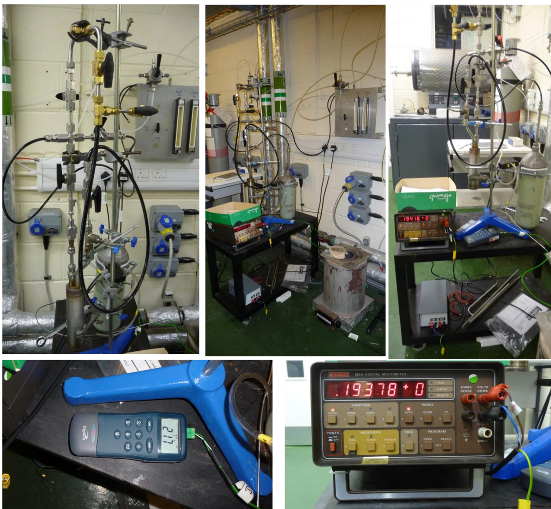
Figure 12-7. Permeameter in use. NB the pressure reading is in Volts, directly from the sensor. The transfer function included in the relevant sensor datasheet was used to convert these into pressures in kPa in an Excel spreadsheet.
