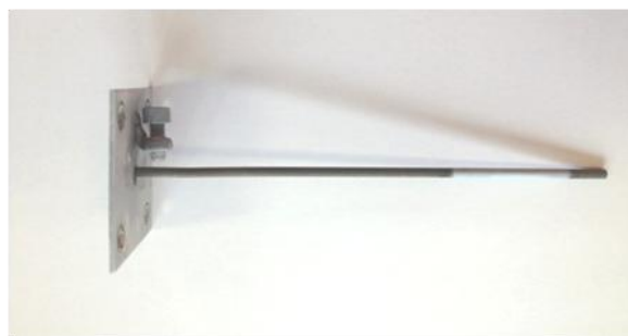
Figure 9-15. EB-PVD updated deposition jig that is both simplified and holds the sample more securely while removing the risk of damage that existed with the previous version.
