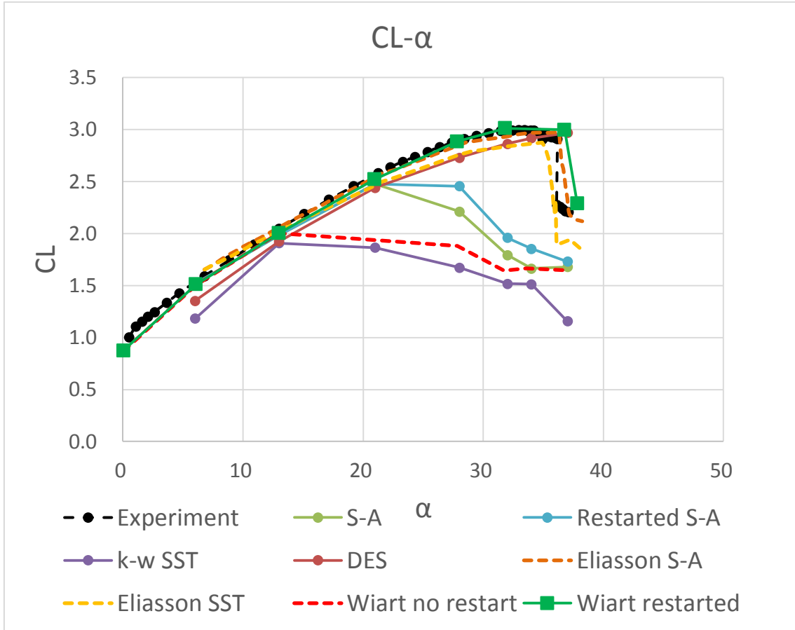
Figure 5.10 Comparison of lift coefficient vs seven various angles of attack for S-A, k-w SST, DES and experimental results
