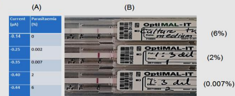
Figure 5: Average amperometric signal of the culture medium supernatant (6% parasitaemia) in 3-fold serial dilution (A). Comparison with Immunochromatographic detection of LDH in serial dilution of culture medium supernatant using optiMAL-IT kit (B).
