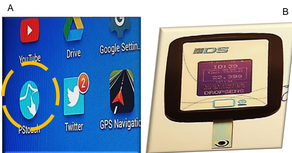
Figure 4-1: PStouch application (A) useful for analysing and up-loading data from remote locations, and DropSens hand-held potentiostat (B).
