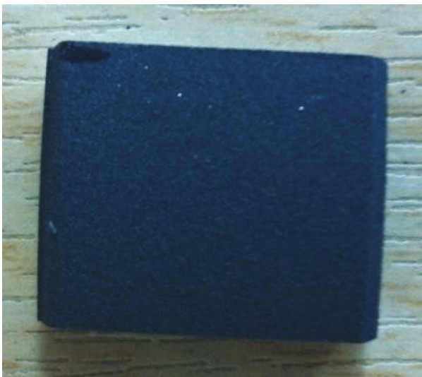
Figure 1. Examples of tube segments used for corrosion exposures, the samples are about 15 mm x 15 mm, with 4 mm thickness.
