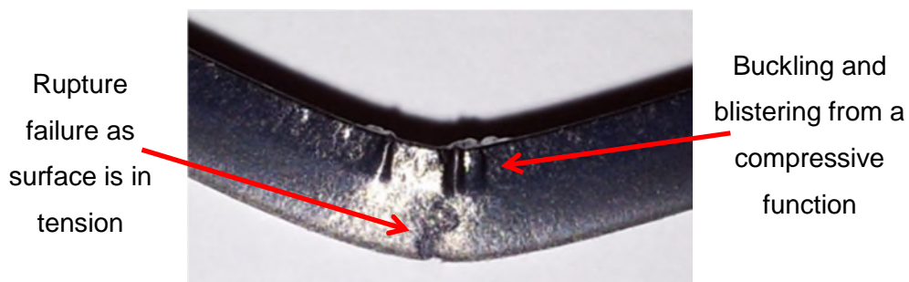
Figure 3-6 showing one of the failed material B specimens from 120°C testing
