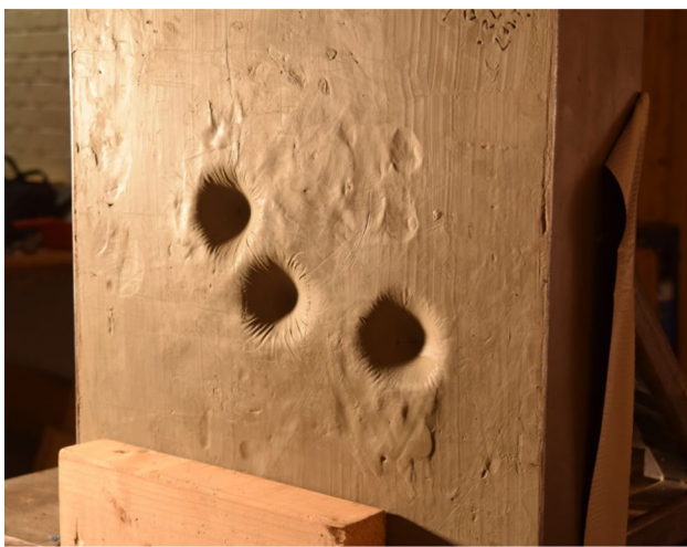
Fig. 6 Back face trauma from 67 ms -1 impact
