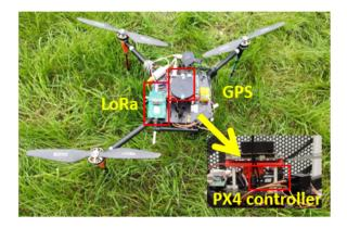
Figure 2. The UAV and its hardware layout.
