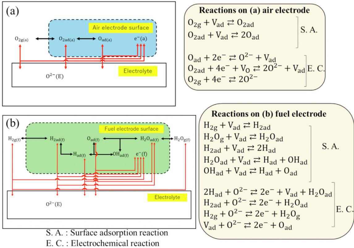
**Fig. 6 – Possible reactions on (a) the air electrode and (b) the fuel electrode, after Hosoi et al. [29]. The subscript “ad” denotes an adsorbed species or an adsorption site. The subscript “g” denotes a gas molecule.**
