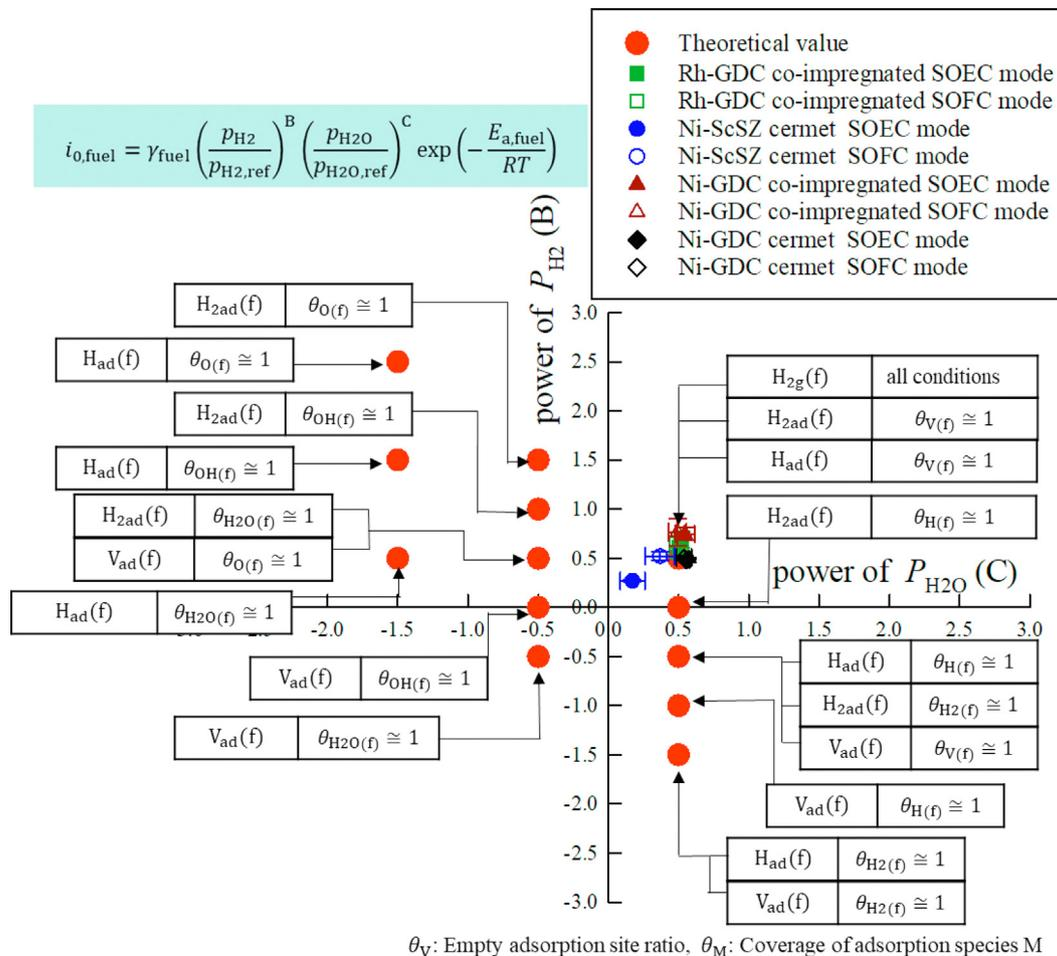
**Fig. 8 – Fuel electrode surface coverage ( $\theta_M$ ) and gas concentration dependence, analyzed using the  $p_{H_2}$  and  $p_{H_2O}$  dependencies compiled by Hosoi et al. [29].**
