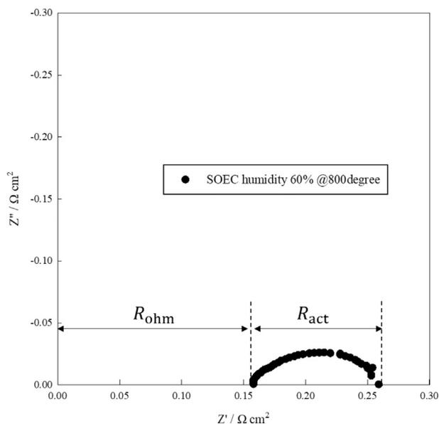
Fig. 1 – - Typical impedance spectrum of an SOEC operated with 60%-humidified  $\text{H}_2$  at 800 °C.
