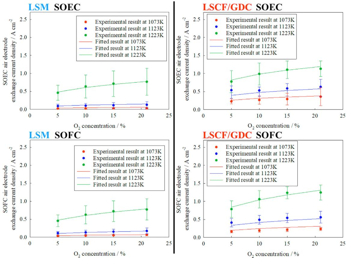
Fig. 2 – Apparent exchange current density of the air electrodes. (Fuel electrode: 3%-humidified hydrogen  $100 \text{ mL min}^{-1}$ ; Air electrode:  $\text{N}_2 + \text{O}_2$   $150 \text{ mL min}^{-1}$  (oxygen concentration: 5%, 10%, 15%, and 21%); Operating temperature:  $800^\circ\text{C}$ ,  $850^\circ\text{C}$ , and  $950^\circ\text{C}$ ).
