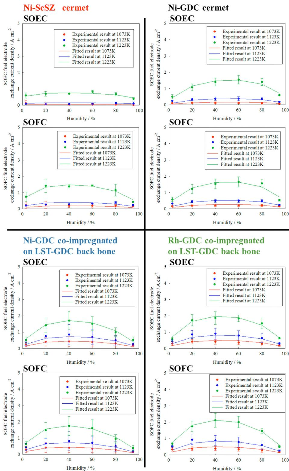
**Fig. 3 – Apparent exchange current density of the fuel electrodes (Fuel electrode:  $\text{H}_2 + \text{H}_2\text{O}$  100 mL min<sup>-1</sup> (humidity: 3%, 20%, 40%, 60%, 80%, and 95%); Air electrode: air 150 mL min<sup>-1</sup>; Operating temperature: 800 °C, 850 °C, and 950 °C).**
