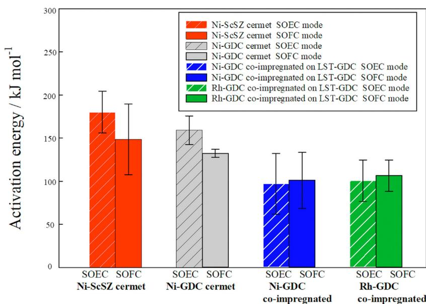
Fig. 5 – Activation energy of the fuel electrode reactions derived using the phenomenological equation (Eq. (4)) for exchange current density of fuel electrodes, with error bars showing standard deviation.
