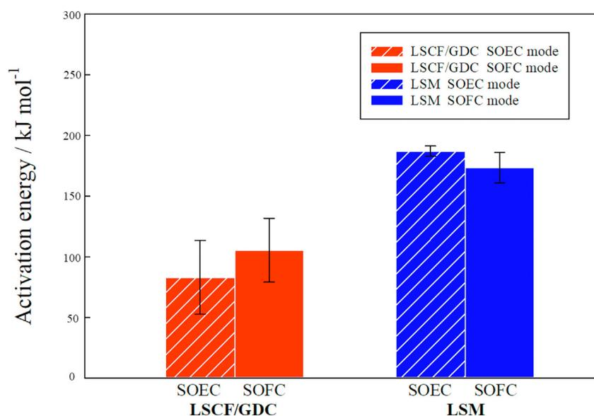
**Fig. 4 – Activation energy of air electrode reactions derived using the phenomenological equation (Eq. (3)) for exchange current density of air electrodes, with error bars showing standard deviation.**
