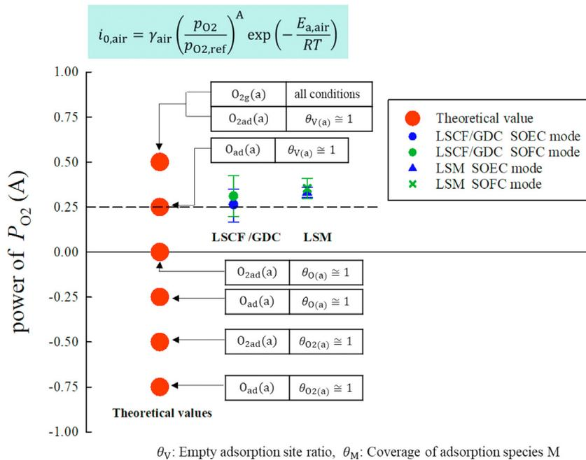
**Fig. 7 – Air electrode surface coverage ( $\theta_{(a)}$ ) and gas concentration dependence, analyzed using the  $p_{O_2}$  dependencies compiled by Hosoi et al. [29].**
