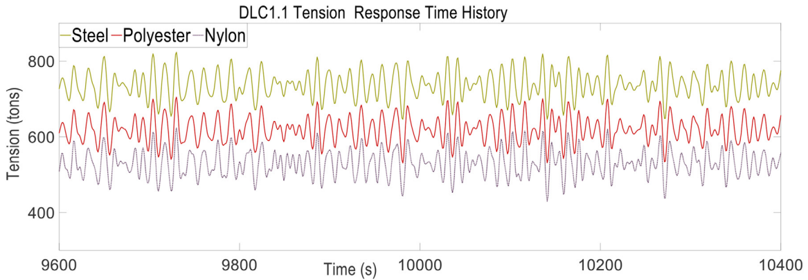
Fig. 25. DLC1.1 Time History of Tension Response for TLB with Nylon, Polyester, and Steel Wire Ropes.
