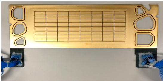
Fig. 6 – Segmented terminals for current distribution analysis.
