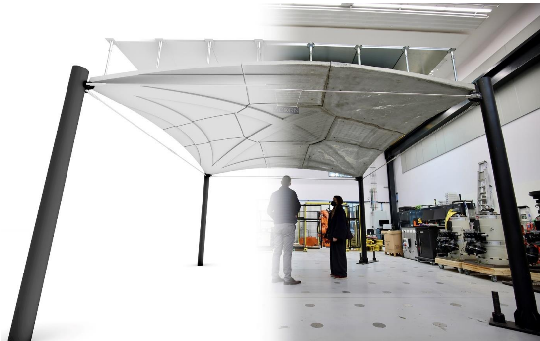
Figure 1 – Left: Render of assembled ACORN thin-shell floor system; Right: Shell standing once assembled on columns with a levelled floor. Photo credit: ©John Orr
