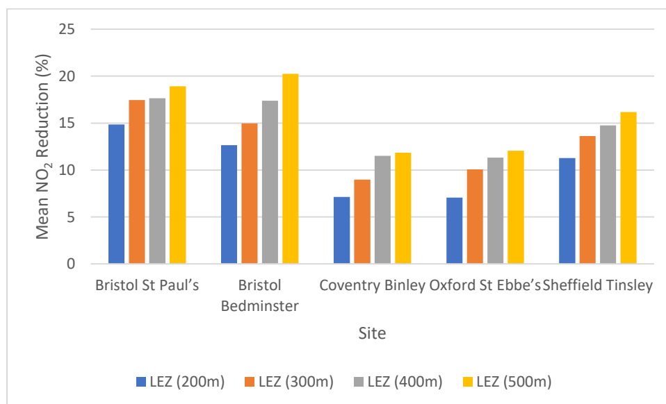
Figure 69 Modelled mean percentage reductions of NO 2 at travel routes due to active travel, anti-idling, rideshare, improved travel routes, and Low Emission Zone implementation at 200m, 300m, 400m, & 500m.
