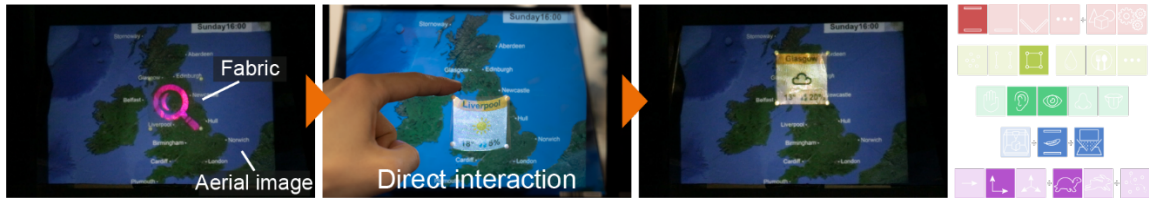
Figure 9: Example E5 showing a geospatial map and presenting the UK weather forecast. The ASKA3D plate provides contextual information about the UK map, while users can directly manipulate the levitated fabric, which shows detailed information about the weather using both visual and auditory modalities.
