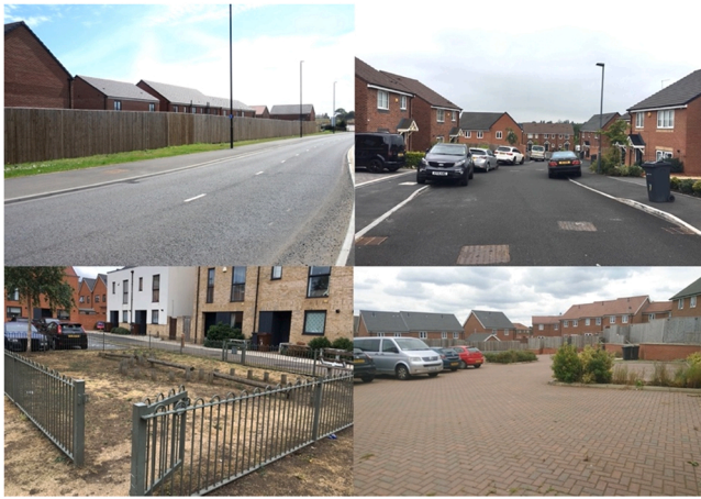
Fig. 37. Low-scoring housing developments scored especially badly in terms of ‘character’ and ‘sense of place’, with architecture that did not respond to the context in which it was located. The worst reported aspects of design included developments dominated by access roads and the poor integration of storage, rubbish bins, and car parking, leading to unattractive and unfriendly environments. All these elements are heavily controlled by generic standards-based codes applied with little thought to holistic place quality (image: Matthew Carmona).
