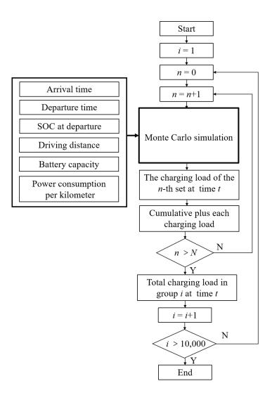
Figure 2. The charging load calculation process.
