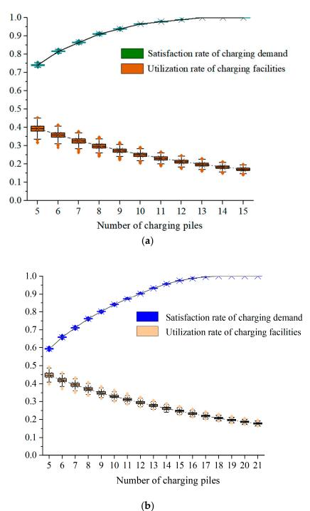
**Figure 5.** Indicator comparison of configuration scheme: (**a**) Design period (Y = 5); (**b**) Design period (Y = 10).
