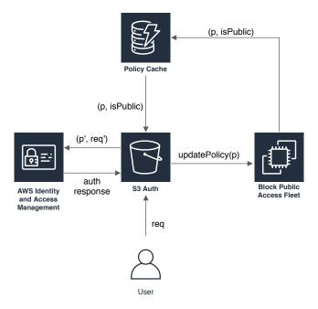
Figure 8: BLOCK PUBLIC ACCESS integration in S3 authorization process.
