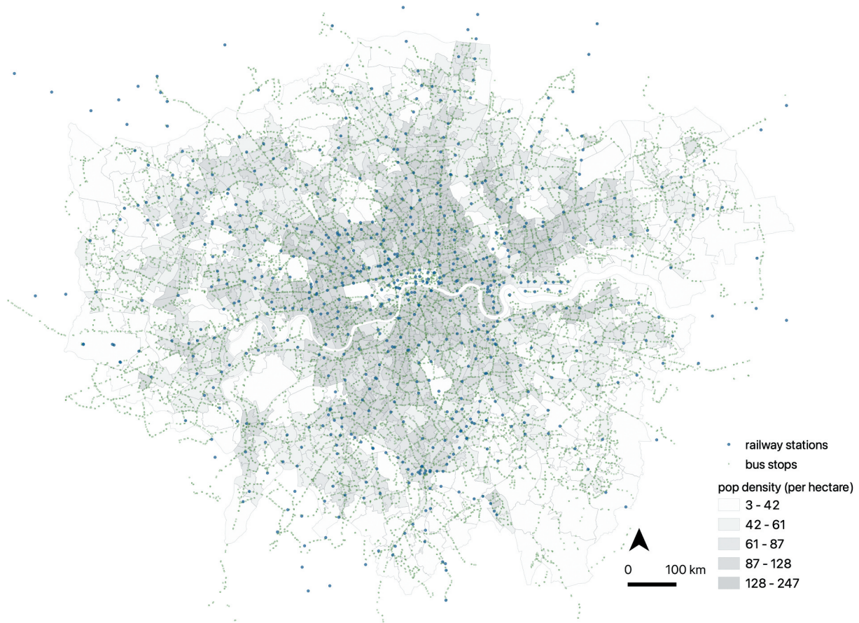
Figure 2. Map of London railway stations and bus stations. A map of London railway stations and bus stops relative to the population density within London. Railway stations are in blue, and bus stops are in green. The population density in gray represents the monocentric distribution of London's residents.
