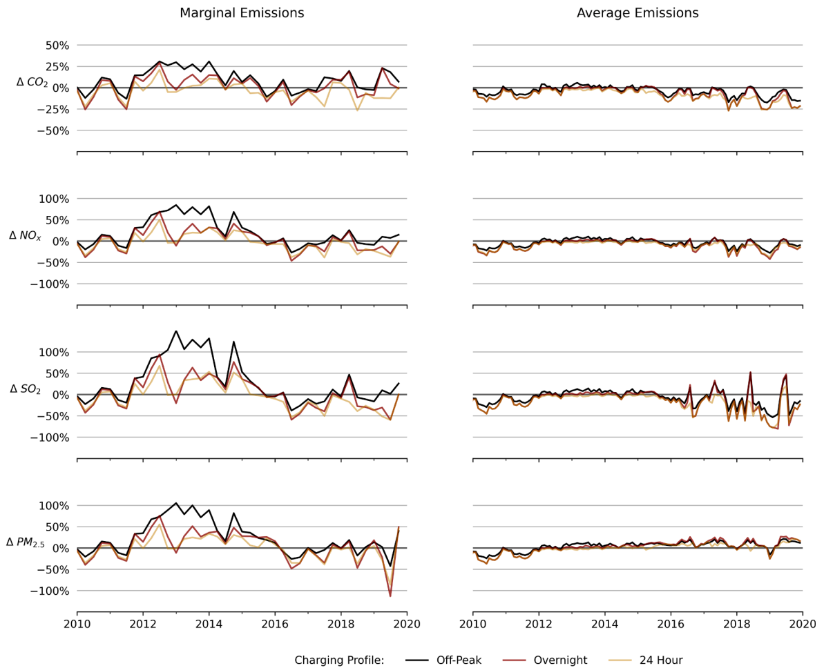
Fig. 9. The relative impact of the different charging strategies on emission rates, compared those from the national average charging profile. These strategies are the average observed off-peak charging pattern of vehicles, and two hypothetical smart-charging profiles (constrained to overnight hours or available 24-hours a day). Marginal emissions (left) are given on a quarterly timescale and average emissions (right) are given on a monthly timescale.
