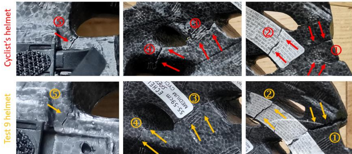
Figure 4. Comparison of cracks between the cyclist's helmet and Test 9 (the numbers mark the cracked regions).
