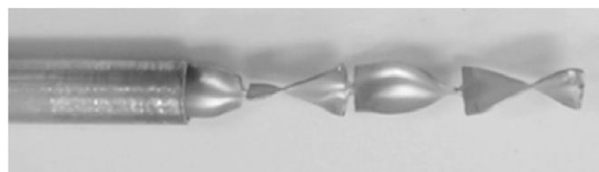
Fig. 5. The tribocharger design employed by Trigwell et al. (Trigwell et al., 2009, 2012) and Quinn et al. (Quinn et al., 2012).
