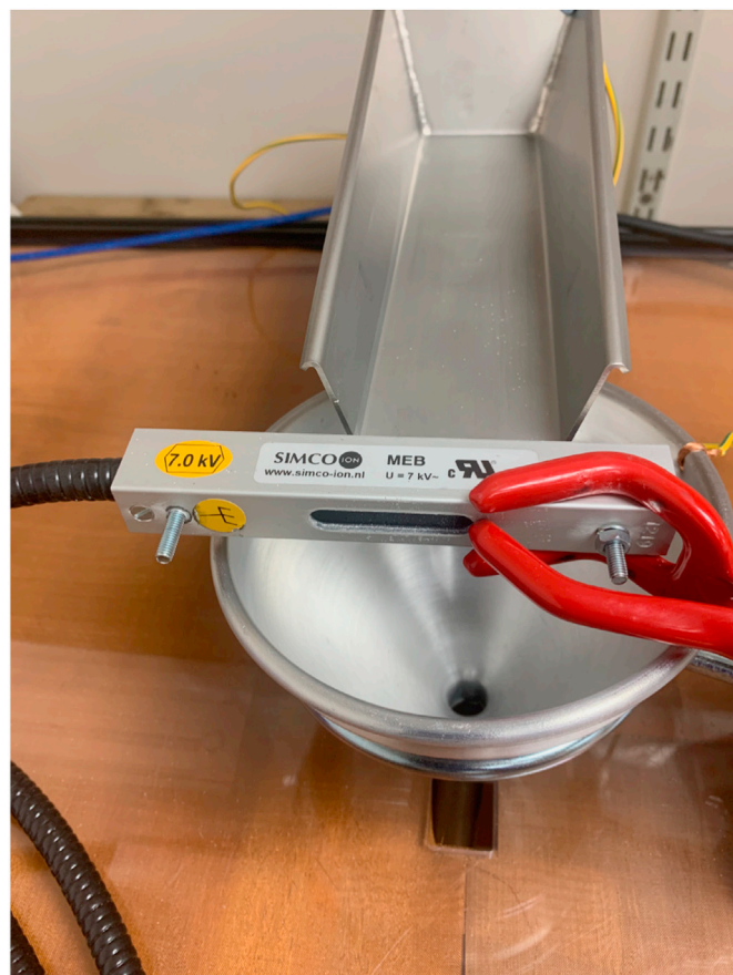
Fig. 4. The feeder arrangement employed in this study. The FT0B linear vibratory feeder conveys particles to the injection point. Here, the Simco-Ion MEB bar emits ions to neutralise any preexisting charge. The falling particles are then guided into the separator by the aluminium funnel.
