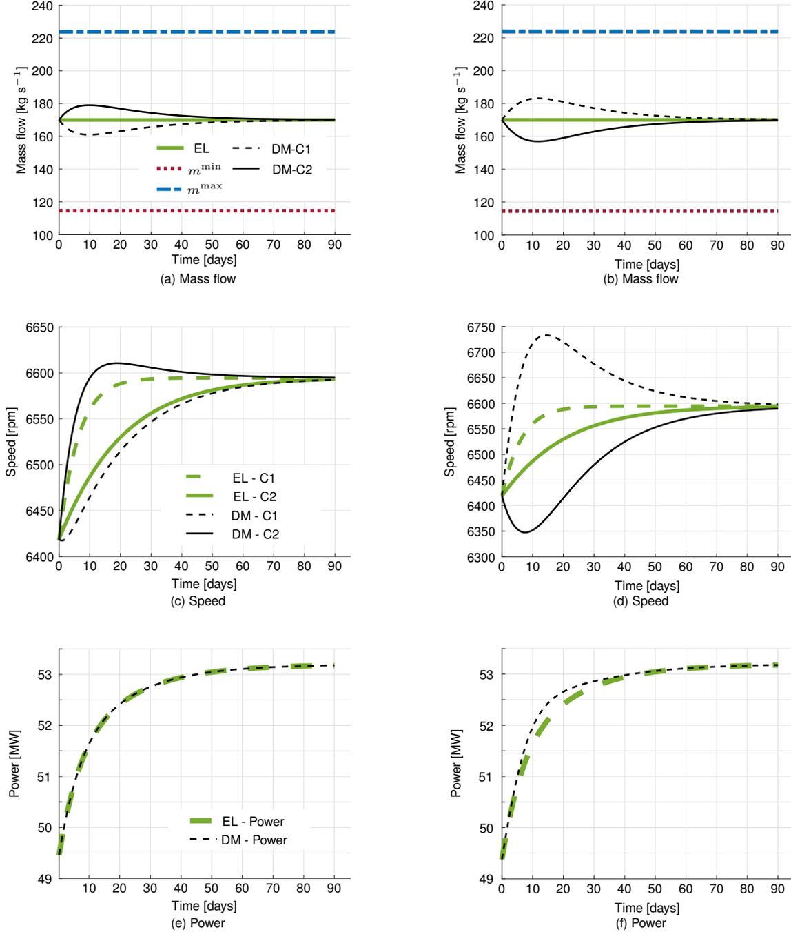
Fig. 3. Process variables for degradation management (DM) in the case of mitigating degradation using  $f_M$  (left column) and intensifying degradation with  $f_I$  (right column) if Compressor 1 (C1) degrades more quickly than Compressor 2 (C2), compared with equal load approach (EL)
