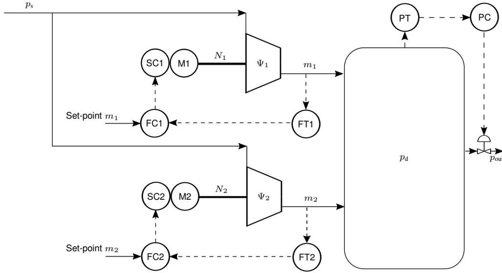
Fig. 1. Compressor station with two compressors connected to the same discharge tank
