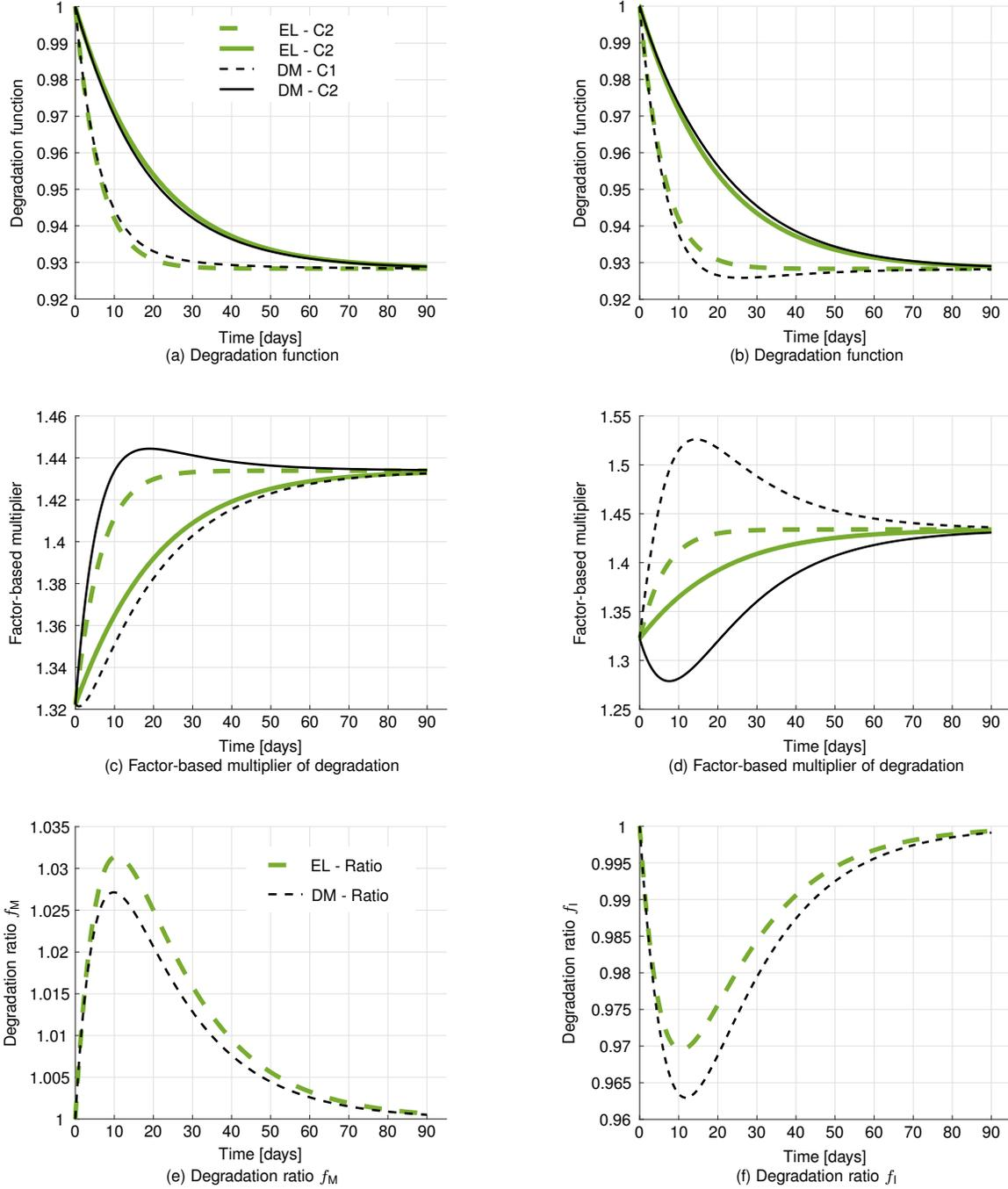
Fig. 4. Degradation variables for degradation management (DM) in the case of mitigating degradation using  $f_M$  and intensifying degradation with  $f_I$  if Compressor 1 (C1) degrades more quickly than Compressor 2 (C2), compared with equal load approach (EL)
