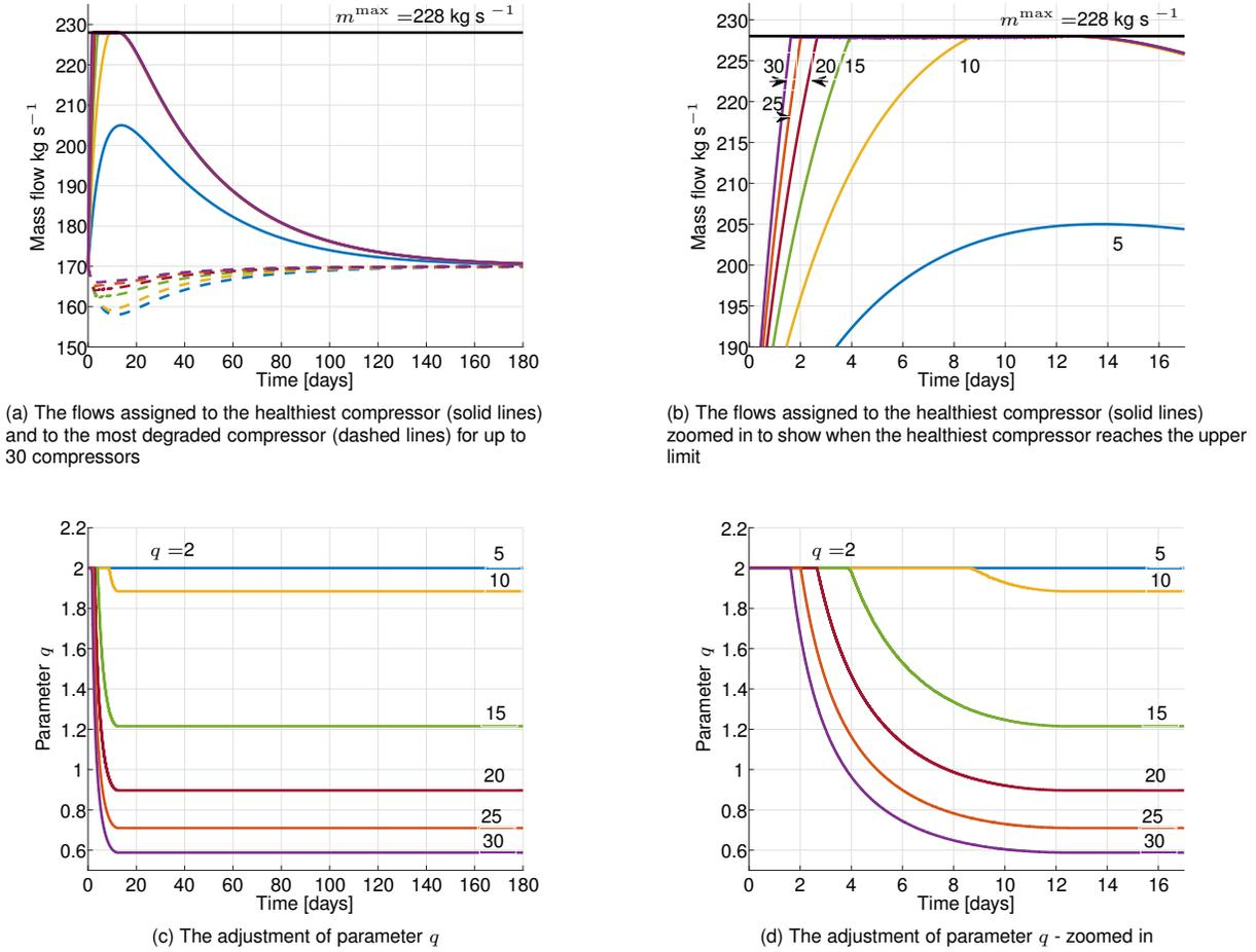
Fig. 12. The flows for the healthiest and the most degraded compressor in the leader strategy with adjusting the parameter  $q$  depending on the number of compressors: 5 (blue), 10 (yellow), 15 (green), 20 (dark red), 25 (orange), and 30 (purple)
