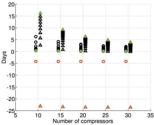
Fig. 13. Number of days gained (+) or lost (-) for compressor stations with 10, 15, 20, 25, and 30 compressors in the collaboration (circles) and the leader strategies (triangles), with the numbers corresponding to the most degraded compressor marked in green and to the healthiest compressor in orange
