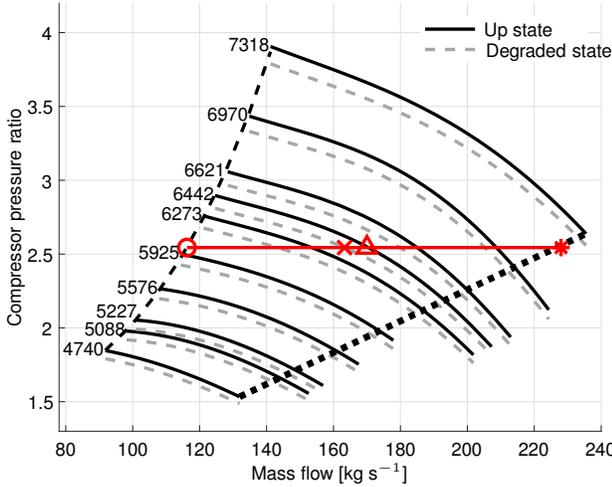
Fig. 2. A compressor map with the pressure ratio as a function of the mass flow and compressor speed in up state and in degraded state. The labels indicate compressor speed in rpm. The data for the compressor map were obtained from [15]
