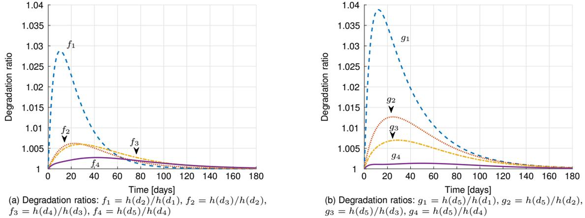
Fig. 9. Degradation ratios for five compressors, obtained using the collaboration strategy (left) and the leader strategy (right)
