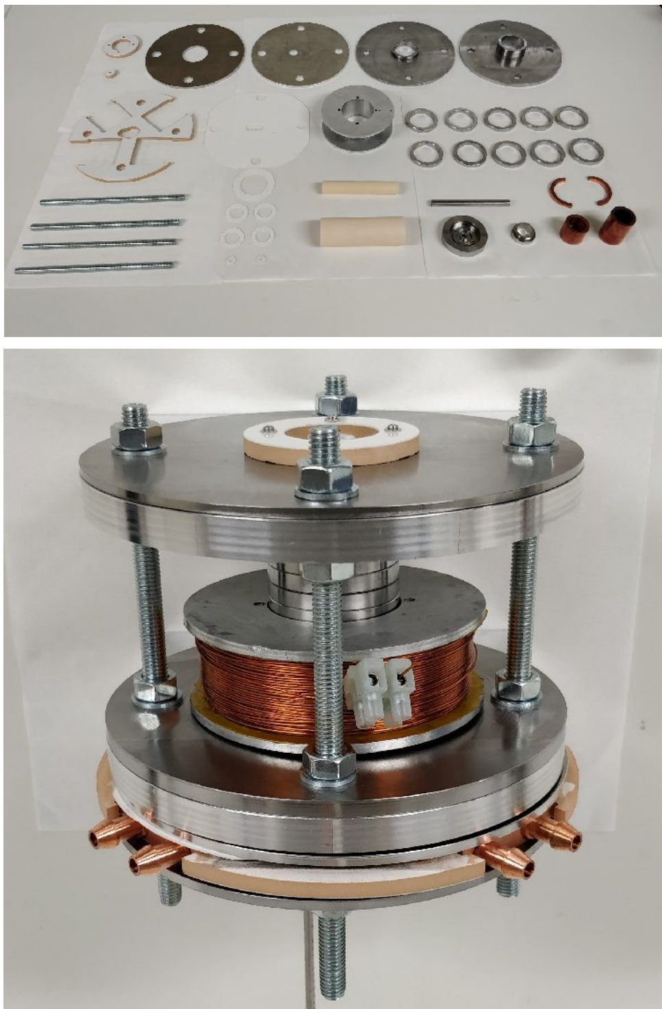
Figure 4.1: The WET-HET disassembled (top) and assembled (bottom). The lower section of the bottom photograph shows the optional water-cooling elements installed on the thruster, which were never used.
