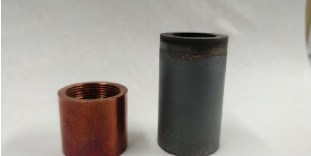
Figure 6.12: A new anode (left) compared to a anode which has seen several hours of operation, which has the anode cap attached (right)
