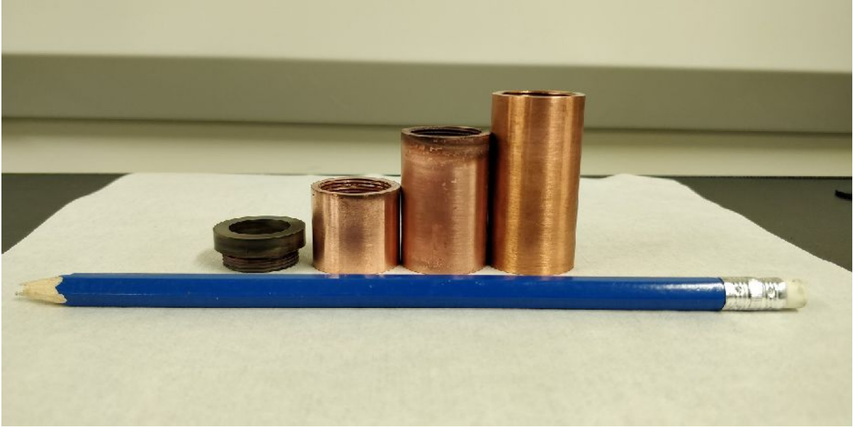
Figure 4.6: The stainless steel anode cap of the WET-HET (left) with three different length copper anodes. Combining the cap with each of the anodes results in a channel depth of 60 mm, 45 mm and 35 mm respectively.
