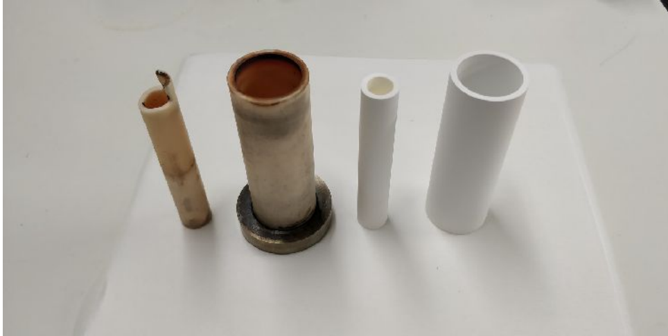
Figure 6.3: The original inner and outer alumina ceramic wall components (left), along with the new boron nitride replacements (right). Note the top of the inner alumina wall (left most) has been heavily damaged from extreme thermal shock.
