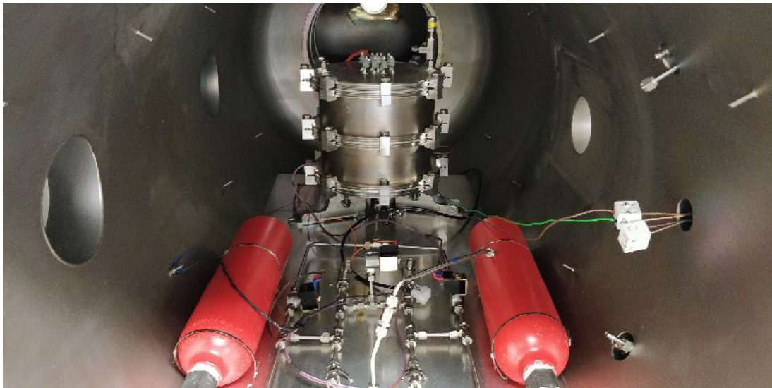
Figure 5.15: The hydrogen supply hardware. This system comprises two plena, several solenoid valves, and an MFC housed within a vessel pressurised to atmospheric pressure. The entire system was housed within the hatch of the Boltzmann Facility.
