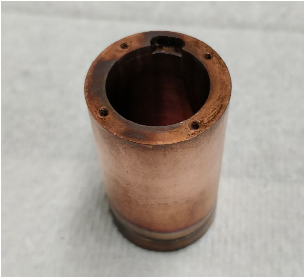
Figure 4.5: The bottom face of the anode showing four tapped holes and the propellant notch which diverts the propellant from the feed-line into the inner section of the anode.
