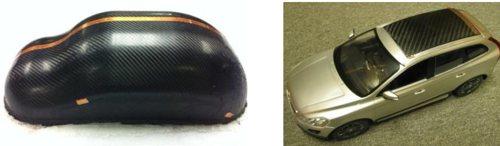
Figure 1 Desktop scale (approximately 30 cm long) structural supercapacitor composite demonstrators in the form of automotive exterior panels able to power LED lights [1]
