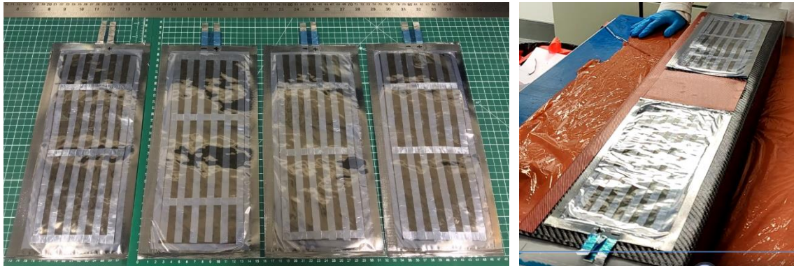
Figure 4 Structural supercapacitor composite cells integrated into the 80 cm long beam
