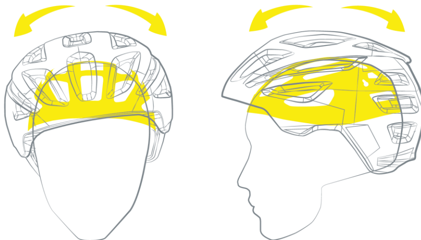
Figure 9 – Multi-directional Impact Protection Systems (MIPS) which is essentially a low friction slip layer (yellow) placed between the rider's head and the outer shell [91].
