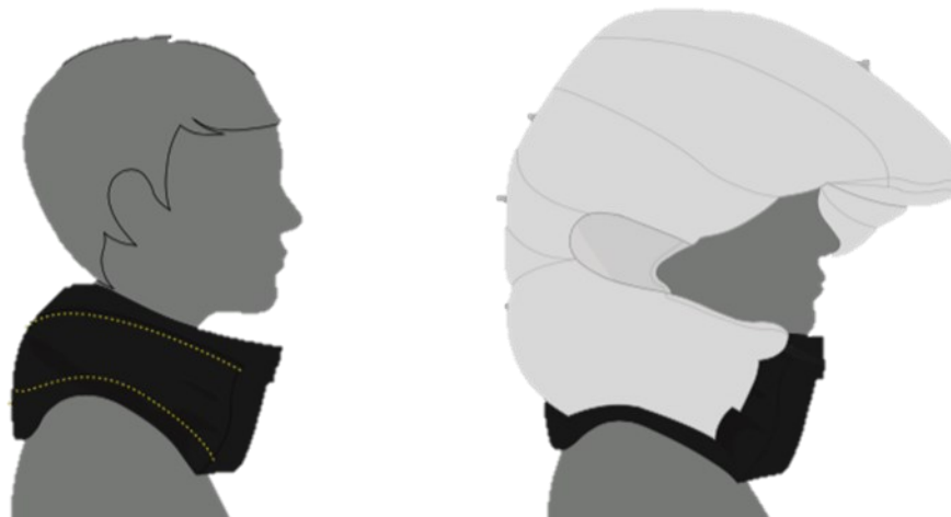
Figure 8 – Hövding airbag in the undeployed (left) and deployed (right) positions [89].
