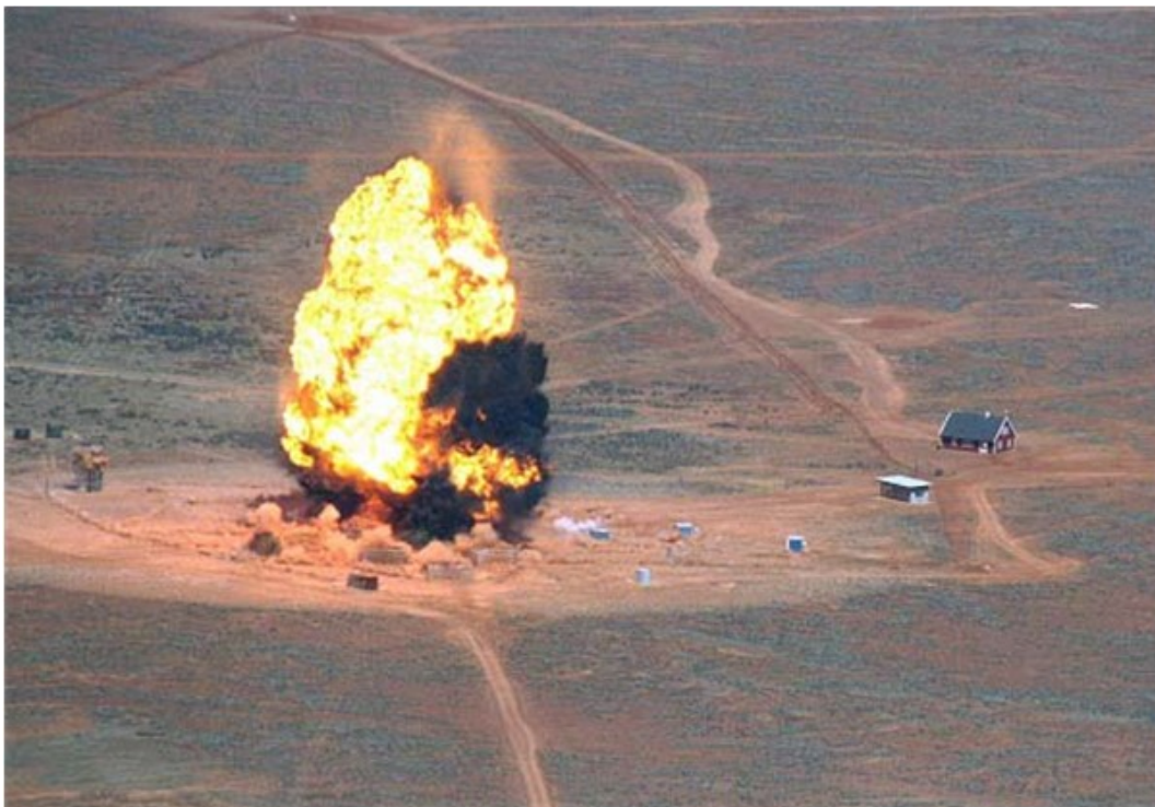
Figure 20: Aerial photograph of 5000 kg trinitrotoluene (TNT) detonated to investigate blast effects (TNO Defence Security and Safety, 2020, figure reproduced with permission).
