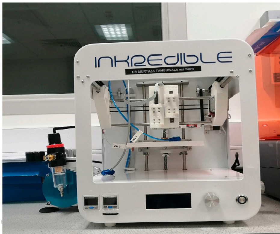
Figure 1. Illustration showing the pneumatic based extrusion Inkredible 3D bioprinter (dual-print head). The bioprinter employed had a UV LED curing system, which assists in bio-printing tissues or any organ model.
