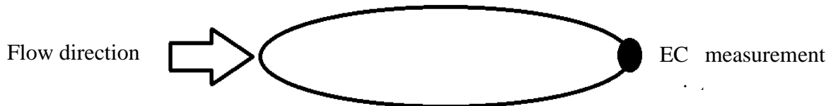
Figure 1.8: Typical shape of EC footprint. The filled circle mark is the measurement point and the arrow indicate the flow direction. The footprint forms upstream of the EC measurement point.
