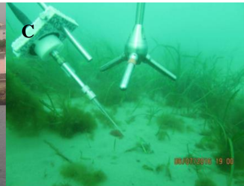
Figure 2.13: Layout of the deployment, A) a schematic of the setup of EC and microprofiler instruments, noting microprofiler is connected via a cable to the dingy which housed the controller and battery (not autonomous). The EC was autonomous (did not require a cable to the dingy). B) The mooring buoy connected to the dingy upon where the control box and battery of the microprofiler lay. C) EC, ADV and oxygen microelectrode surrounded by seagrass. D) Microprofiler oxygen and temperature sensors in situ surrounded by seagrass.
