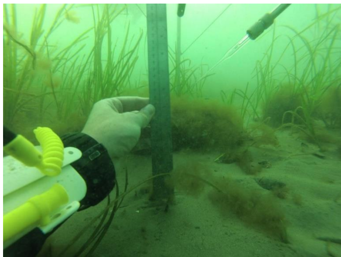
Figure 2.10: Photo taken in situ demonstrating the height of the oxygen microelectrode above the seabed. A rule was used to measure the height ensuring no sinkage of the lander occurred which may have led to the ADV entering a weak spot.
