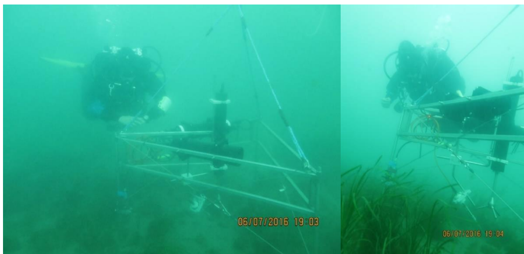
Figure 2.9: Diver checking the location of the EC instrumentation in-situ at Cawsands. This was not possible at L4 due to the depth and harsh environment therefore, a camera set-up was utilised.
