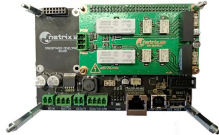
Fig. 4. High-voltage converter on the board of the control module
