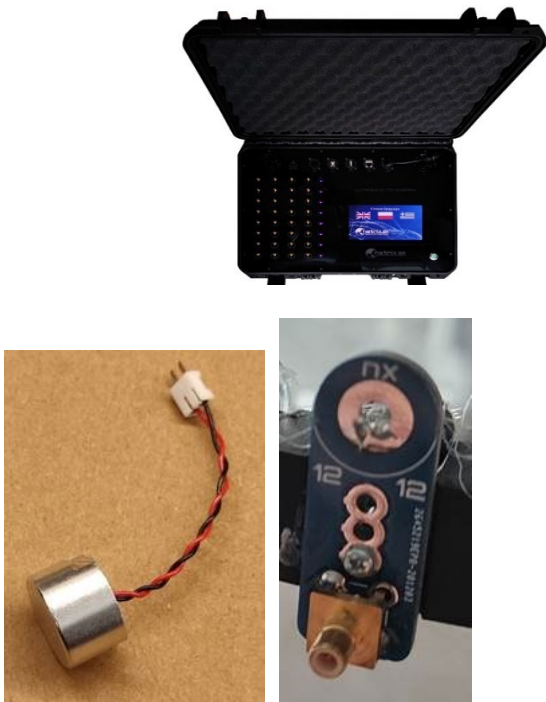
Fig. 2. UST tomograph and the UST transducer
