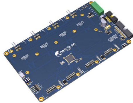
Fig. 3. 3D model of the ultrasound card
