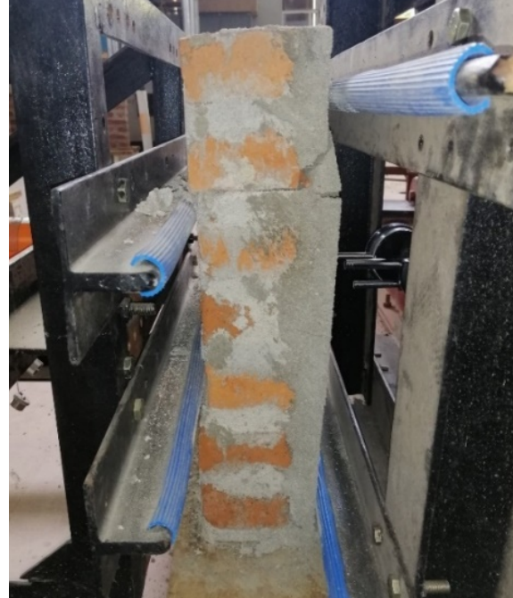
b) typical failure in shear zone of geogrid-reinforced wall
