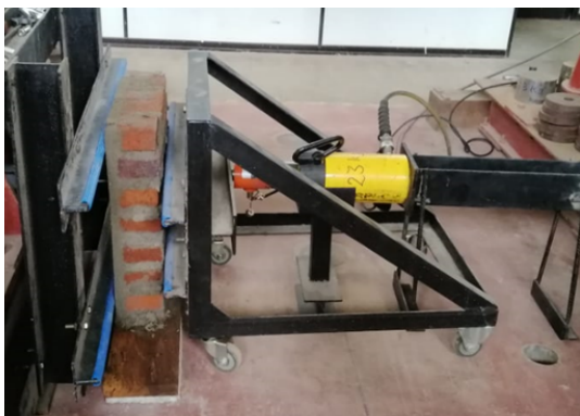
a) Parallel to bed joint flexural test (BE EN 1052-2:2016)
