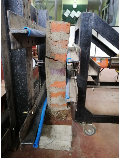
a) parallel bed joint flexural test failure of saturated unreinforced plastered wall
