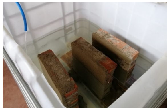
b) 24-hour immersion of panels prior to saturation tests
