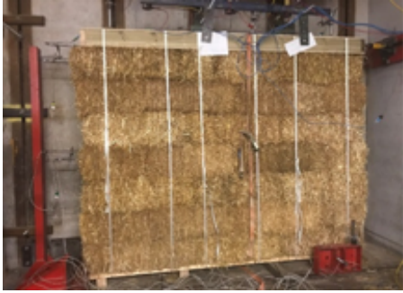
Figure 10 Unplastered wall in-plane racking load test set-up (L:3000mm; W:450mm; H:2300mm)
