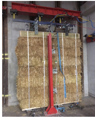
Figure 6 Unplastered two-bale straw bale vertical load test set-up (L:2000mm; W:450mm;H:2300mm)
