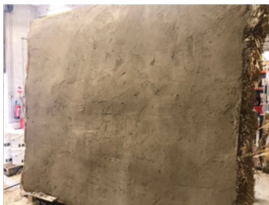
Figure 5 Lime plaster coat
