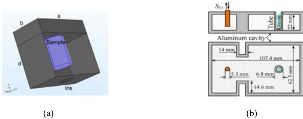
Figure 3.6 Rectangular cavity: (a) sample inside waveguide; [80] (b) sampled in a one-open-end tube [82]
