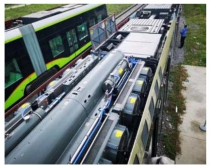
Hydrogen tank and Ballard fuel cell system on CRRC-Sifang light rail https://blog.ballard.com/fuel-cell-trains
