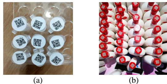
Fig. 1: Multi-QR codes detection scenarios. (a) and (b) present the application of multi-QR codes detection in the medical test tubes for COVID-19 testing and goods warehousing, respectively.
