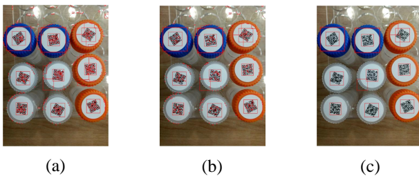
Fig. 7: The results of SDSM and ASSM. (a) shows the bounding boxes. (b) and (c) show the results of the bounding boxes processed by SDSM and ASSM.
