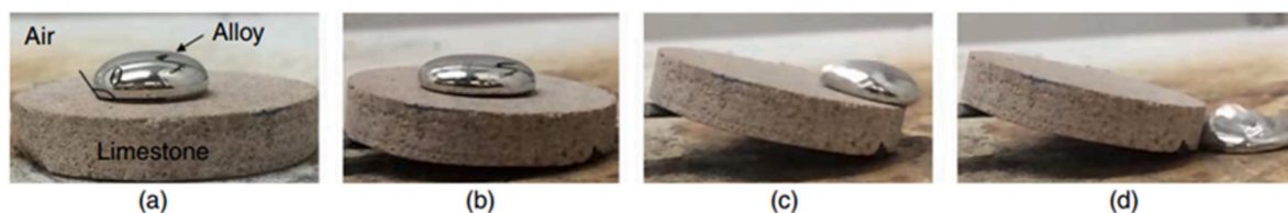
Fig. 14. Illustration of the non-wetting characteristics of molten BiSn alloy on preheated limestone surface (a - molten alloy on flat rock surface; b - d, molten alloy on increasingly tilted rock surface). Adapted from (Zhang et al., 2020).
