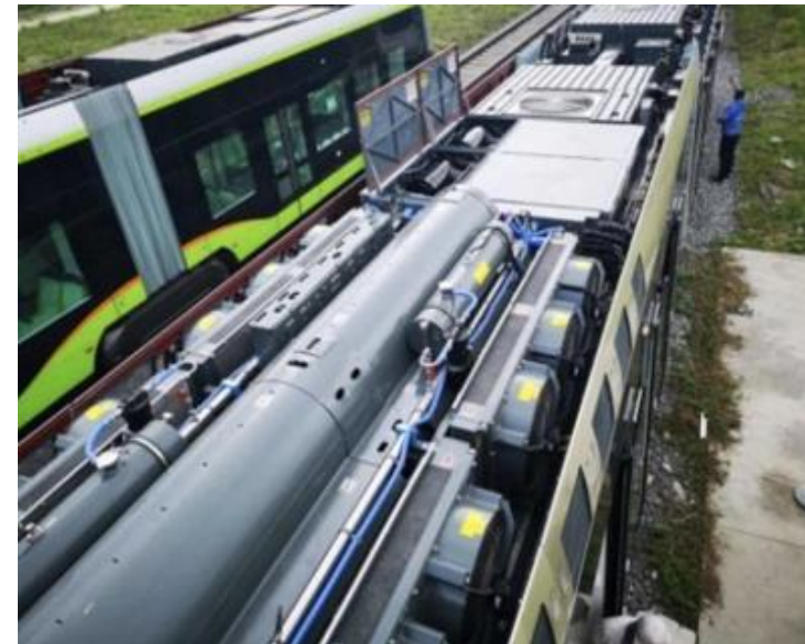
Hydrogen tank and Ballard fuel cell system on CRRC-Sifang light rail https://blog.ballard.com/fuel-cell-trains
