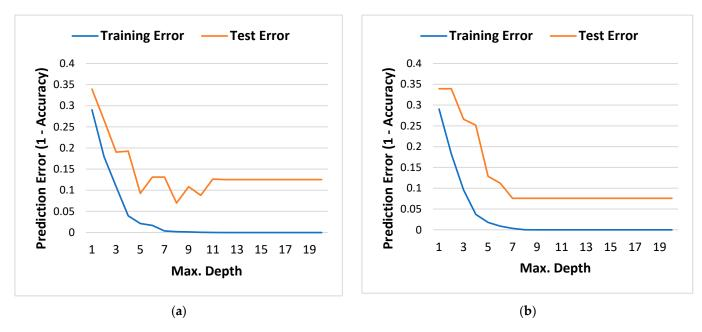
Figure 5. Model training error vs. test prediction error. (a) DT prediction error; (b) RF prediction error.
