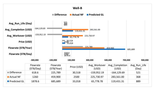
Figure 10. Well-B production and cost difference of actual and predicted AL.
