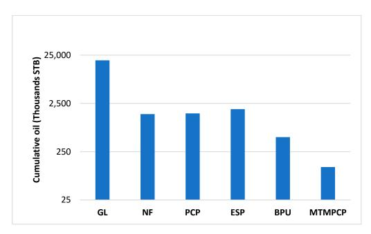
**Figure 3.** Cumulative oil produced by each AL according to IOR and EOR.
